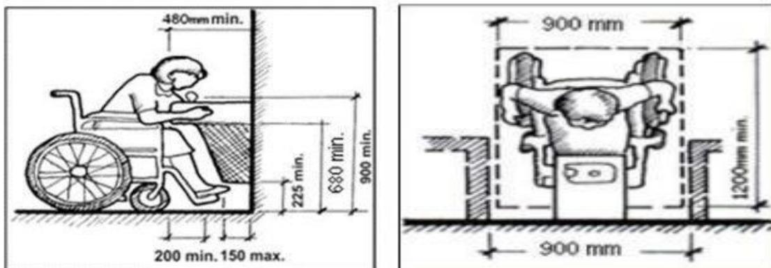
Fig.-10 Standard design principles of Drinking Water Facilities
