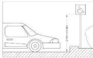
Fig - Vertical sign at designated accessible parking spaces
