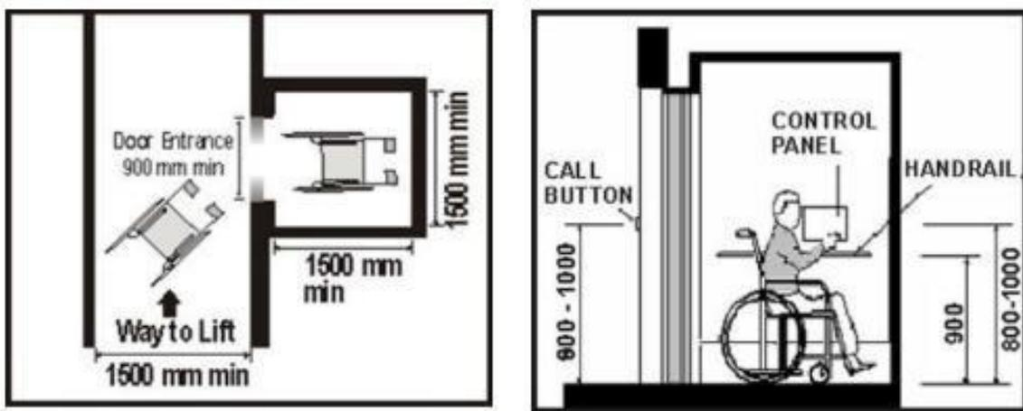
Fig.-7 Lift Dimensions and placement of its control panel
