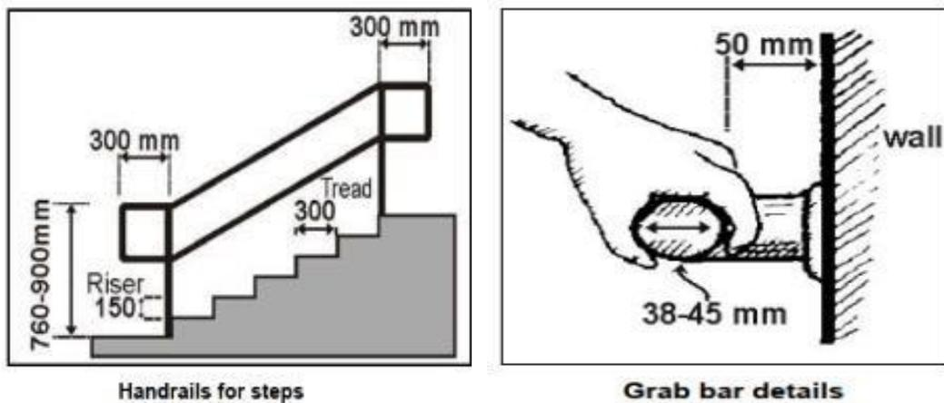
Fig.-8 Dimensions of Staircase and placement of the Hand rail
